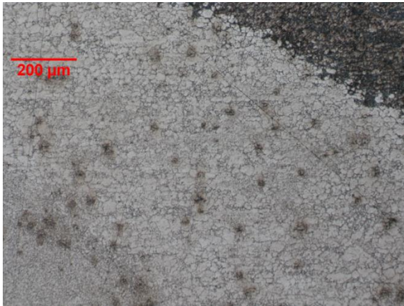
Figure 7: Angle welded at 400 rpm 3 ipm, and 9000 lb forge force showing granular HAZ in the middle. Top right shows parent material, bottom left shows weld nugget.
