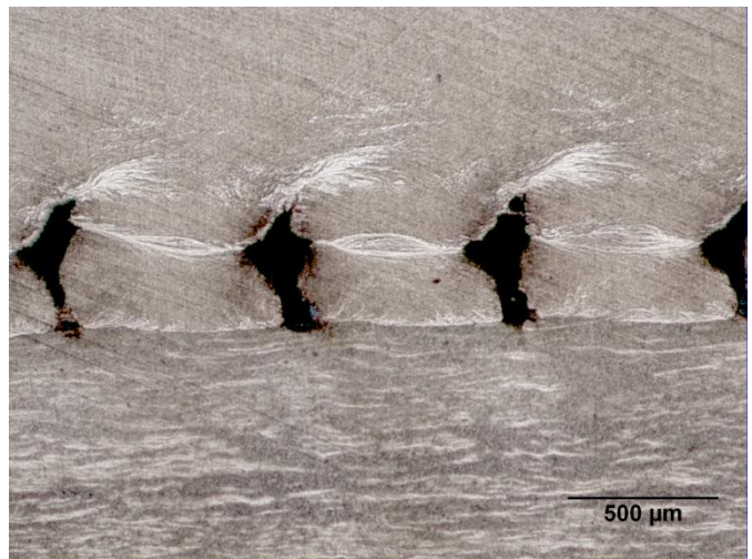
Figure 12: Periodic voids in sample welded at 12 ipm seen from the side of the weld.
